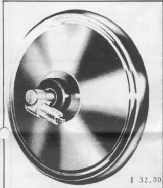
The HARTWIG FRONT WHEEL DRIVE consists of a modified VDO Angle Drive, either type # 210.011 (1:1) or # 210.061 (6:1) with steel shafts and rugged ratio gears, seated in a felt-sealed, dustproof ball bearing, press-fitted into a precision machined high impact flange of ERTALON plastics.
