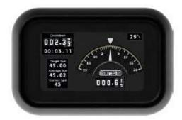
Within average speed stages, an audible warning is triggered at 30 seconds, 15 seconds, and then a ten second countdown to better allow the driver to synchronise themselves to the control timing.
